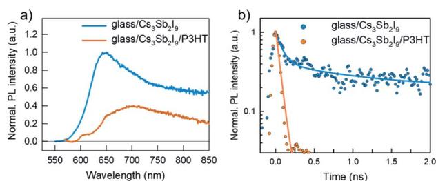
Fig. 4 (a) Steady-state photoluminescence (PL) spectra and (b) time-resolved PL (TRPL) decays of glass/ $\text{Cs}_3\text{Sb}_2\text{I}_9$  and glass/ $\text{Cs}_3\text{Sb}_2\text{I}_9$ /P3HT films, excited at 405 nm (excitation intensity  $\sim 20 \text{ nJ cm}^{-2}$  and time resolution  $\sim 60$  ps). Solid lines show the results of fitting with a bi-exponential function:  $I_{PL(t)} = A_1 \times e^{(-t/\tau_1)} + A_2 \times e^{(-t/\tau_2)}$ .
