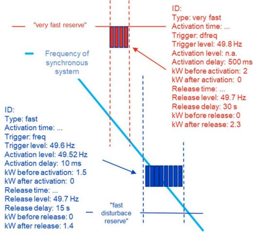
Fig 2. An example of FFR activation patterns and thresholds.
