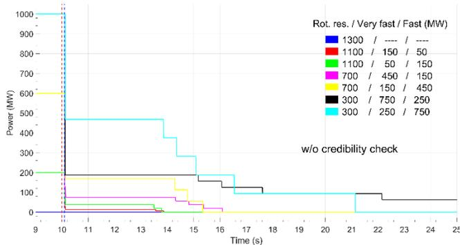
Fig. 8. Load shedding response after 1300 MW production loss with different amounts of ACFRs w/o credibility check.
