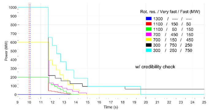
Fig. 10. Load shedding response after 1300 MW production loss with different amounts of ACFRs w/ credibility check.
