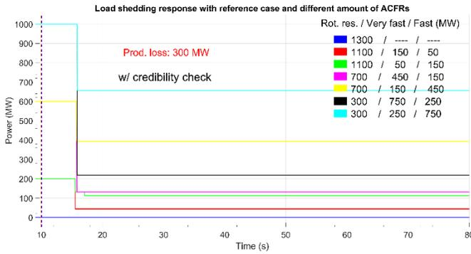
Fig. 12. Load shedding response after 300 MW production loss with different amounts of ACFRs w/ credibility check.
