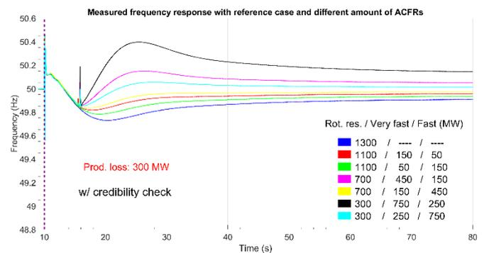
Fig. 11. Measured system frequency response after 300 MW production loss with different amounts of ACFRs w/ credibility check.
