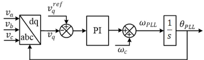
Fig 4. Schematic representation of the SRF-PLL-based frequency measurement.
