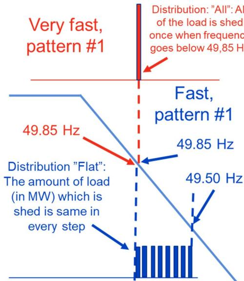
Fig. 5. Load shedding pattern and parameterization of the Type 1 for Very fast and Fast reserves.
