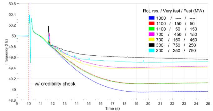
Fig. 9. Measured system frequency response after 1300 MW production loss with different amounts of ACFRs w/ credibility check.
