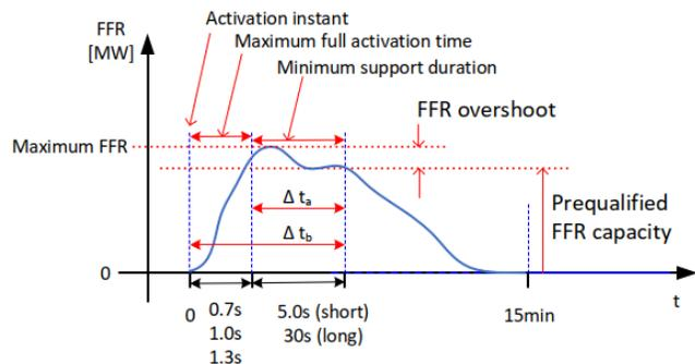
Fig 1. Requirements for FFR activation [1].
