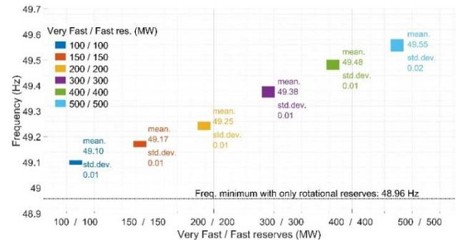
Fig. 6. Results of shedding pattern and parameterization on frequency minimum with different load shedding schemes.
