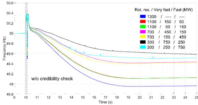
Fig. 7. Measured system frequency response after 1300 MW production loss with different amounts of ACFRs.
