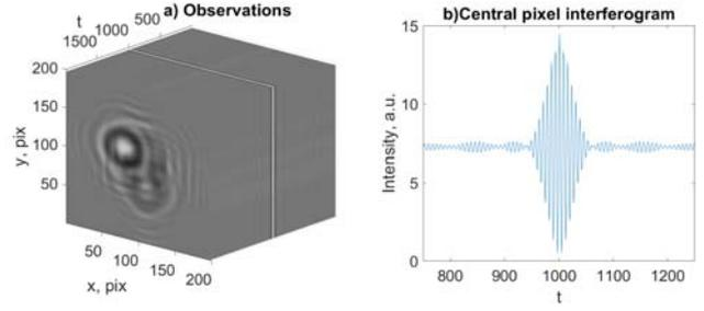
**Fig. 3.** (a) 3D noisy intensity observations: diffractive data cube  $Z_t$ ; (b) The intensity distribution for the central pixel of the 3D data cube  $Z_t$  as a function of the slice number  $t$ .
