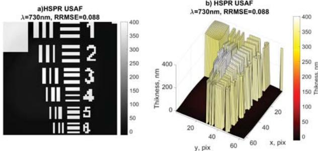
**Fig. 2.** Reconstruction of the object thickness obtained from the phase retrieval for the wavelength  $\lambda = 730$  nm.
