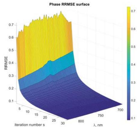
**Fig. 4.** RRMSE of the object phase reconstruction depending on iteration number  $s$  and wavelength  $\lambda$ .
