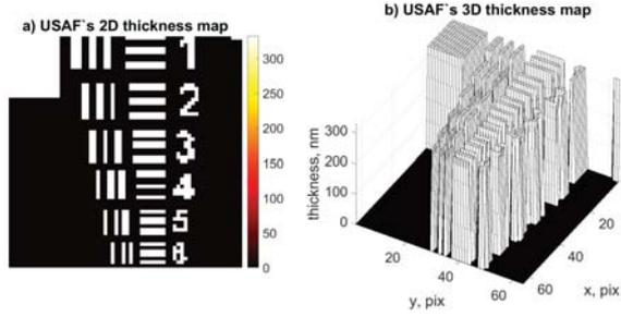
**Fig. 1.** Thickness of the transparent phase object: 2D (a) and 3D (b) images.
