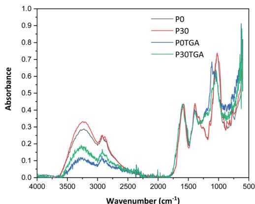
Fig. 3 FTIR spectra of films conditioned at 40% RH and 23 °C (P0, P30) and directly after being heated from 30 to 150 °C at a rate of 5 °C  $\text{min}^{-1}$  (P0TGA, P30TGA). The IR absorbance was normalized to the peak starting from *ca.* 1570  $\text{cm}^{-1}$  to *ca.* 1600  $\text{cm}^{-1}$ , which includes the amide I peak.
