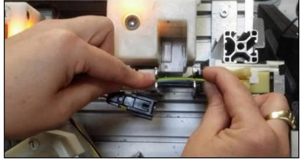
Fig 5. A worker assembling the harness, picking the cable with the Right hand using the Palmar Pinch (9) grasp and routes the cable with the Left hand using the stick (29) type grasp
