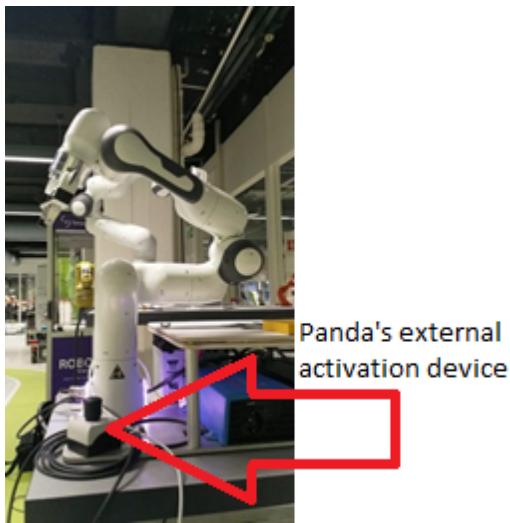
Figure 2: - Collaborative robot Franka Panda. It has seven degrees of freedom and is 119 centimeters tall.
