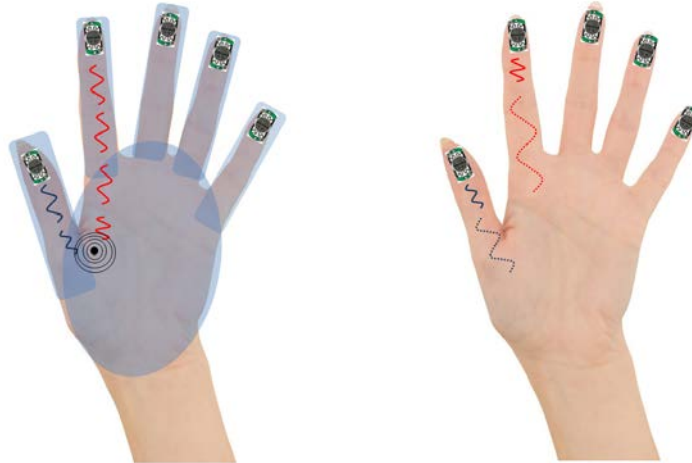
Fig. 2. Internal design of the Liquid Mediation layer, Actuator placement and signal attenuation for the two gloves.
