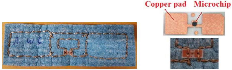
Figure 2. Ready-made embroidered sensor tag (left) and close look of the microchip and antenna-microchip interconnection (right).
