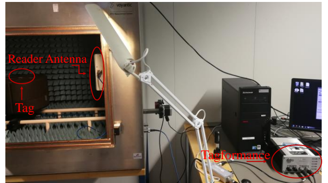
Fig. 5. Measurement set-up in an anechoic chamber.
