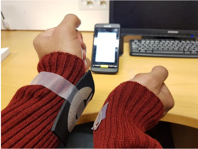
Fig. 7. Initial comparison of the three different wrist antennas: Antenna on a substrate is taped into a shirt wrist and an ID ring is taped into the other wrist of the shirt.
