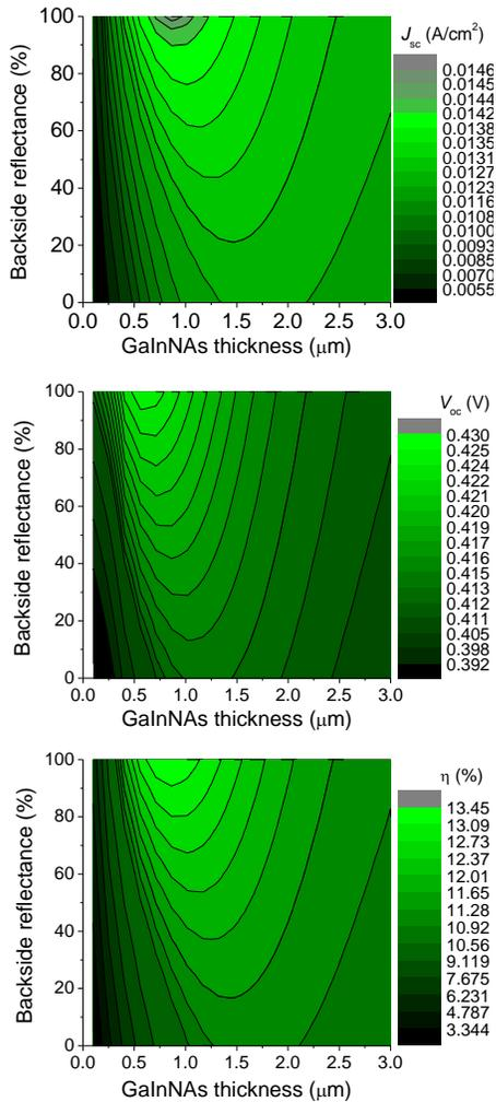
Fig. 4  $J_{sc}$ ,  $V_{oc}$  and  $\eta$  of a n-i-p solar cell as functions of reflectance of the diffuse reflector and GaInNAs thickness.
