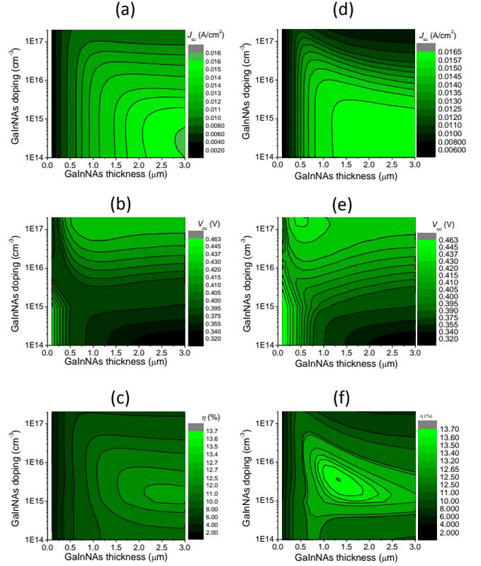
Fig. 3. (a)-(c) Modeled GaInNAs n-i-p solar cell characteristics without backside reflector. (d)-(e) Modeled GaInNAs n-i-p solar cell characteristics with a 95% diffuse backside reflector.
