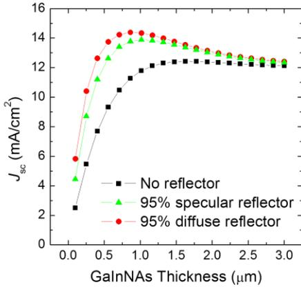
Fig. 2. Comparison of calculated  $J_{sc}$  vs. GaInNAs thickness for solar cells with and without reflectors. The simulation parameters for the cell are taken from [14]. The background doping level of the GaInNAs layer is  $2.2 \times 10^{16} \text{ cm}^{-3}$ .
