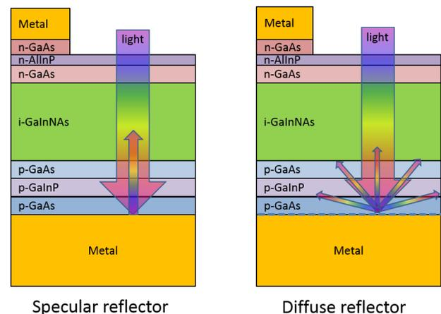
Fig 1. Generic test structures for the GaInNAs back surface reflector solar cell with different reflector types.
