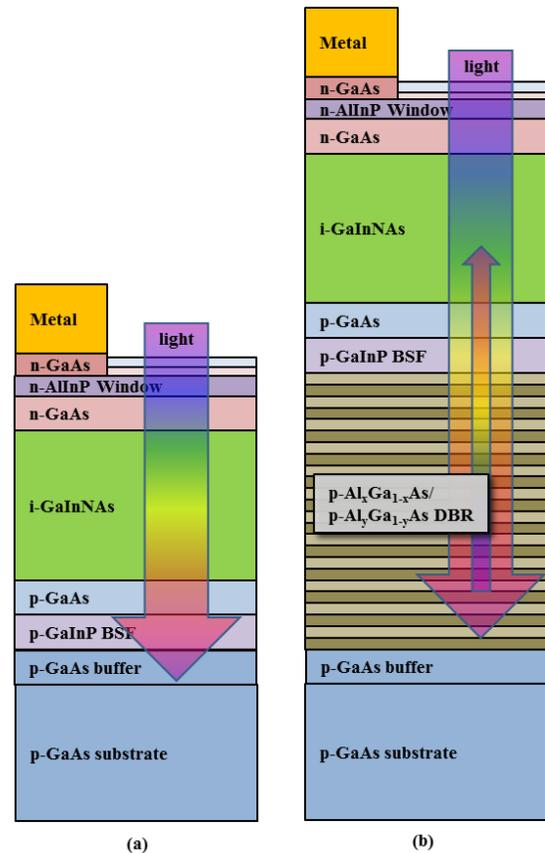
Fig 1. Generic test structures for the GaInNAs solar cells with AlInP window and GaInP back surface field (BSF) layers: (a) single junction GaInNAs solar cell and (b) GaInNAs solar cell with a DBR back reflector.
