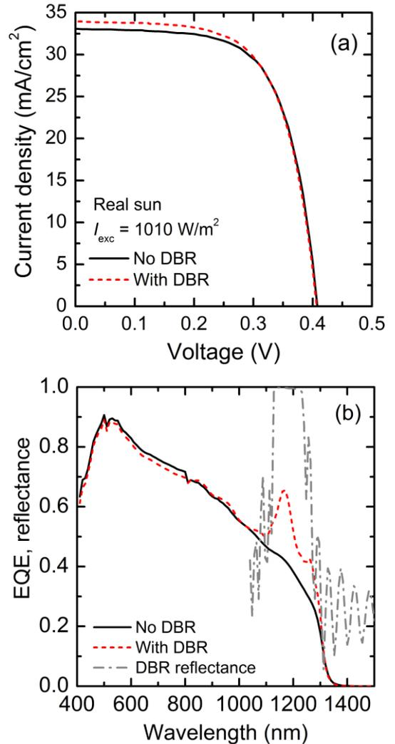
Fig. 2. (a) Measured LIVs from GaInNAs solar cells with and without DBR reflectors. (b) EQE and reflectance values for GaInNAs solar cells with and without DBR reflector showing the improvement of photocurrent in the GaInNAs junction.
