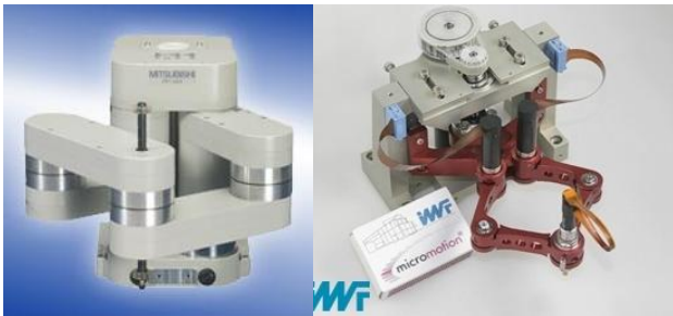
Figure 2 On left, Mitsubishi RP robot [7] and on right, Parvus robot (image from http://www.sfb516.tu-bs.de/english/t2/t2_en.html ). Images are in different scales.
