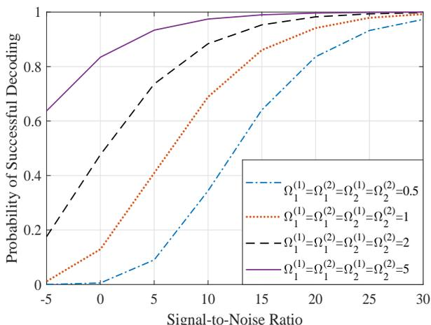
Fig. 11. Performance comparison of split file caching-aided NOMA for the cost function given in (44) with SNR, for different values of the parameters  $\Omega_1^{(1)} = \Omega_1^{(2)} = \Omega_2^{(1)} = \Omega_2^{(2)} = \Omega$ , and  $m_1^{(1)} = m_1^{(2)} = m_2^{(1)} = m_2^{(2)} = 1$ .
