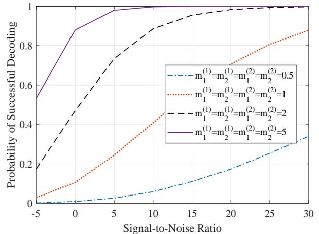
Fig. 12. Performance comparison of split file caching-aided NOMA for the cost function given in (44) with SNR, for different values of the parameters  $m_1^{(1)} = m_1^{(2)} = m_2^{(1)} = m_2^{(2)} = m$ , and  $\Omega_1^{(1)} = \Omega_1^{(2)} = \Omega_2^{(1)} = \Omega_2^{(2)} = 2$ .
