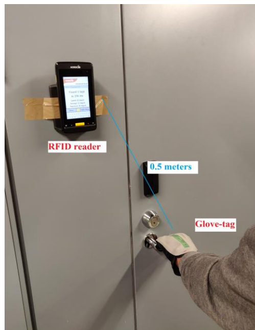
Fig. 11. Practical evaluation of glove-tags: identification (top) and access control (bottom).
