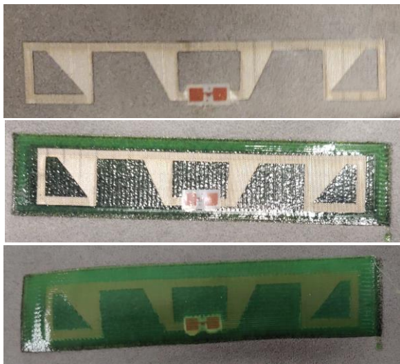
Fig. 4. Fabrication steps of glove tags: Electro-textile antenna was ironed either directly onto the glove surface (top) or onto a 3D-printed structure that was printed onto the glove surface (middle). After IC attachment, both types of ready glove-tags were coated with 3D-printed structures (bottom).
