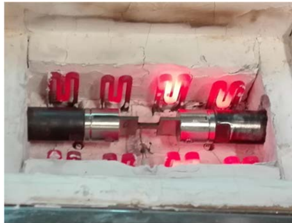
Fig. 2. Resistors system for furnace heating.
