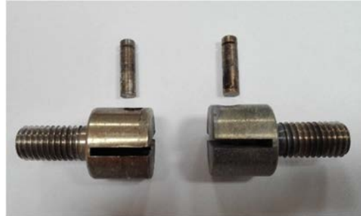
Fig. 1. a. Ti6Al4V samples geometry, Madrid; b. Clamp designed to attach the specimens. All dimensions are in mm.
